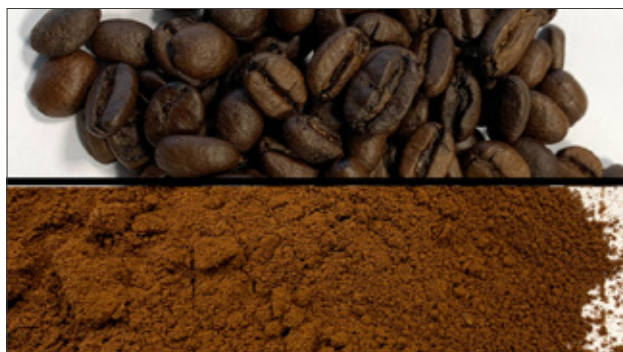
Grinding of coffee beans at a sample cooling temperature of -60°C for natural substance analysis.
